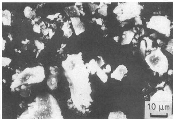
Figure 11 Scanning electron micrograph of the sintered pyrophyllite-potassium carbonate system.
