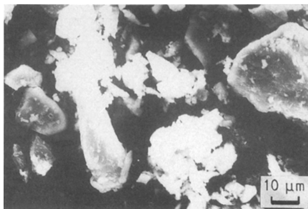
Figure 12 Scanning electron micrograph of the sintered pyrophyllite-sodium carbonate system.
