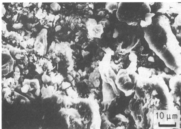
Figure 10 Scanning electron micrograph of the sintered pyrophyllite-lithium carbonate system.
